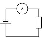
Figure 10.4: An ammeter should be connected in series in a circuit.
