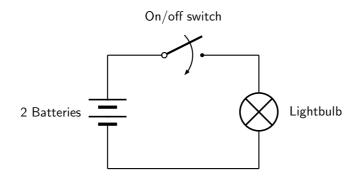
Figure 10.2: Circuit diagram of an electric torch.
