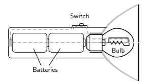
Figure 10.1: Physical components of an electric torch. The dotted line shows the path of the electrical circuit.
