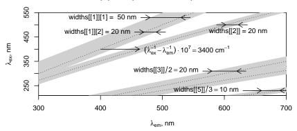
In this example, a much larger portion of the anti-Stokes area is removed near the first order Rayleigh scattering signal than in the Stokes area. This can be useful to get rid of undesired signal where no fluorescence is observed on some spectrometers. The second and third order scattering signal areas are automatically scaled 2 and 3 times, respectively.
