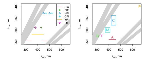
Positions of the peaks and the areas used to determine the fluorescence indices of an EEM. The Rayleigh and Raman scattering areas for both 1st and 2nd diffraction orders are shown in grey, assuming a width of  $\pm 20$  nm and a Raman shift of  $3400~{\rm cm}^{-1}$ . The tolerance interval of  $\pm 1$  nm is invisible at the scale of the figure.
