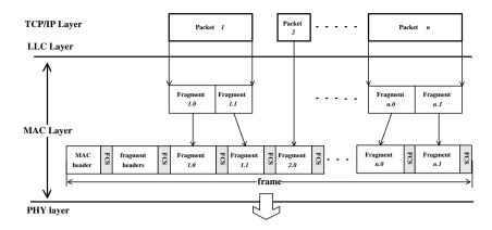
Figure 1. The Aggregation with Fragment Retransmission (AFR) scheme.
