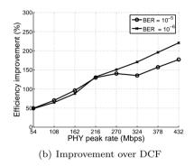
Figure 4. Simulation for CBR traffic with different PHY data rates. Parameters are listed in Table 3.
