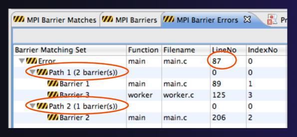
Double-click on a row in Barrier Errors view to find the line it references in the code
